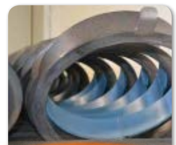
Freehanded rubber coating on nearly every surface
